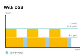
to monitor the required dew point suppression, the dryer saver cycle starts and stops the dryer when the compressor has stopped, minimizing energy use and protecting the air system from corrosion.
