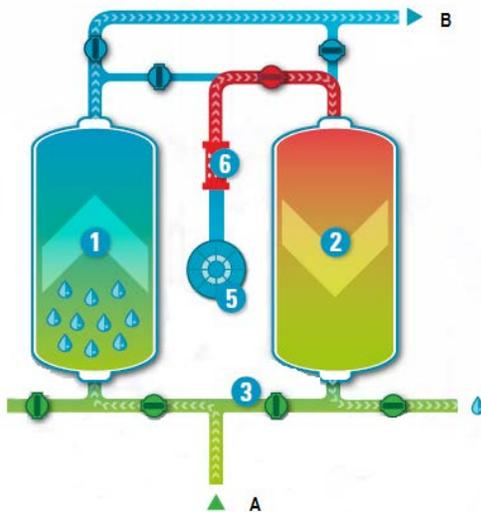
With BD dryer, the blower (5) takes ambient air and blows it over the external heater (6). The heated air is then sent through the saturated desiccant (2), forcing the absorbed moisture out, from top to bottom. Cooling, Zero Purge: After the heating, the hot tower desiccant is cooled. Cooling is done by sending air from the hot vessel (2) over a cooler and back into the hot tower, from bottom to top.
