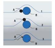
(1) Impaction occurs for relatively large particles. Due to the large inertia of a heavy particle, it does not follow the air streamline but instead travels straight ahead and collides with the glass fiber.
